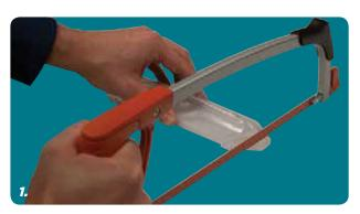
Using a hacksaw, cut the ends of the shell to the appropriate size for your cable.
