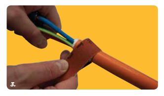
Abrade the cable to the dimensions in the installation instruction and clean with the supplied cleaning wipe.
