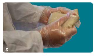
Mix the two parts of the resin together thoroughly.
